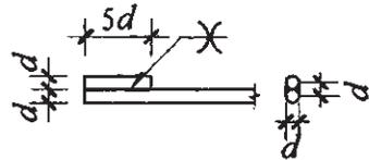
(c) 末端一侧贴焊锚筋
