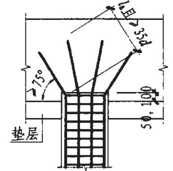
桩顶纵筋在承台内的锚固构造
